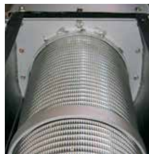
Screw presses from Läckeby Products are fitted with an inspection hatch for the press unit, and replaceable press pipes.
