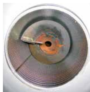
Interior view of the press pipe in Wedge Weir and spiral in black material, S355J0.
